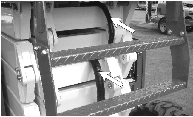
Figure 7.11 - Wiring Harness in the Scissor Stack
