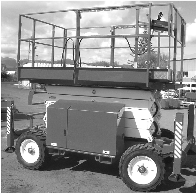
Figure 10.1 - Correct Stowed Position
