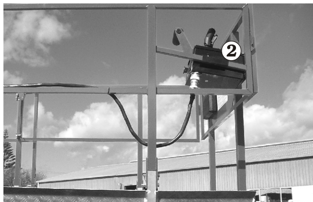
Figure 6.1.2 - Control Box Location, Platform Position
